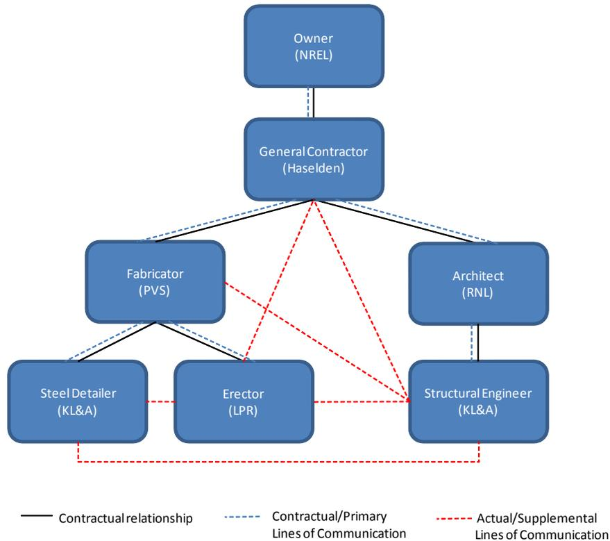
**Figure 1. Contractual Arrangement for the Structural Steel Delivery of the NREL Project.**
