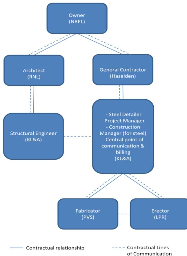
**Figure 2. Proposed Integrated Steel Delivery Model.**
