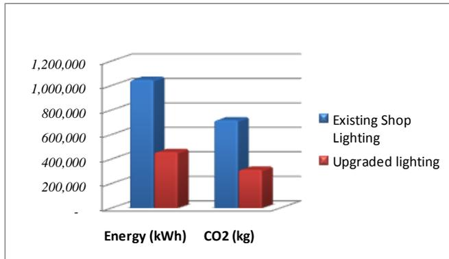
Figure 6. Fabrication Shop Lighting Upgrade.
